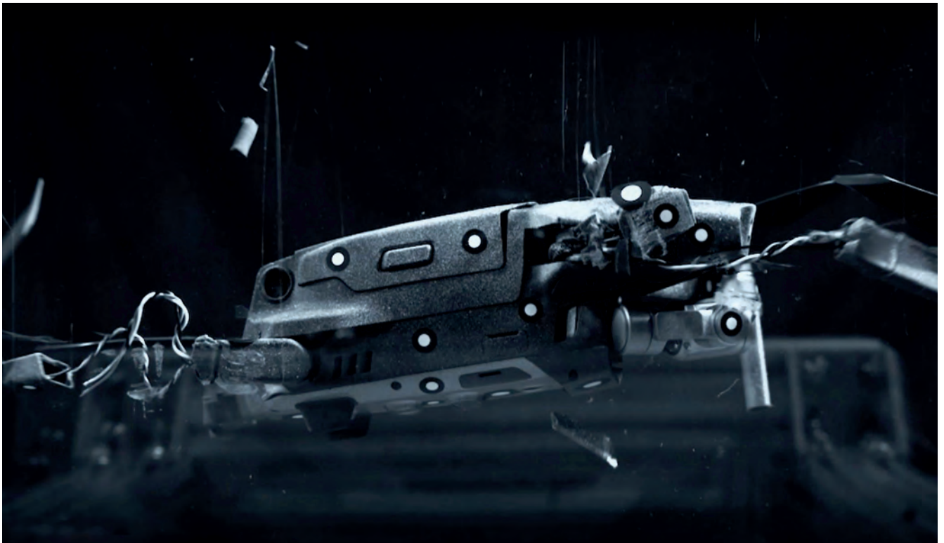
Collision of a drone with a windshield-type structure.
