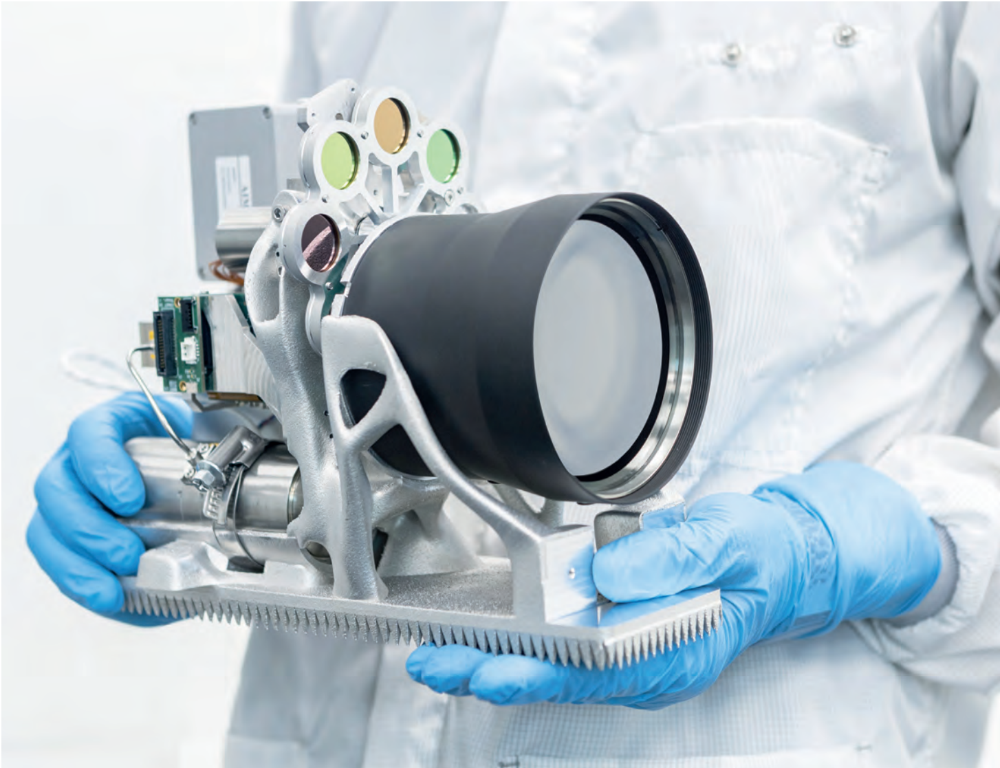
ERNST infrared payload integrated with detector-cooler unit, filter wheel and optics in the additively manufactured optical bench.
