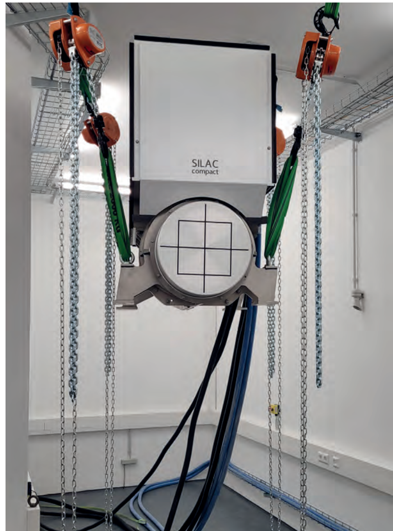
Linear accelerator Linac in test operation during the technical expert inspection.
